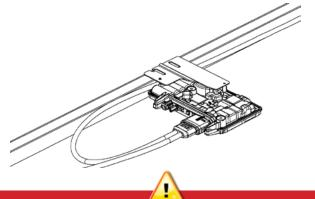
WARNING: Install sealing caps on all unused AC connectors as these connectors become live when the system is energized. Sealing caps are required for protection against moisture ingress.
