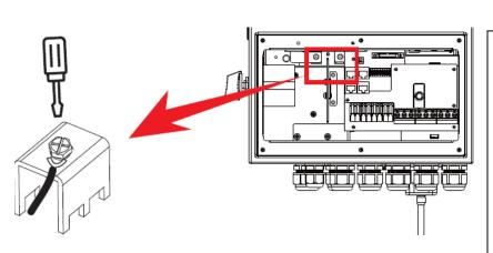
Sol-Ark 5K-1P-N is a <u>48V</u> system. Do NOT wire the battery bank to any other nominal voltage.
