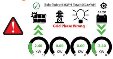
If the Sol-Ark screen shows the above error, there is a phasing issue with your wiring, and it may cause overload faults (F18, F26, F34) even with the Load breaker **off** and **WILL CAUSE DAMAGE** if **left unchecked**.
