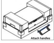
top of the IQ System Controller 2 enclosure until it clicks into place. Check that the handle is secure.
