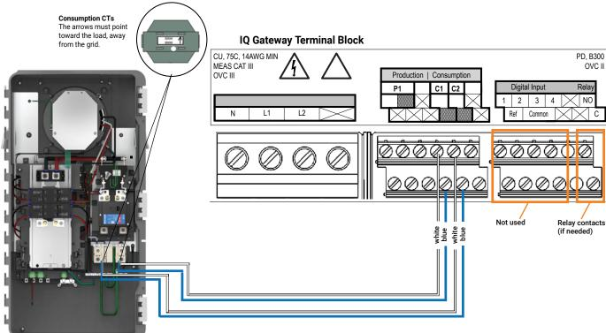
F) For Production as well as Consumption/PCS CTs, you must apply the following label to each CT when the system is configured to use PCS-based current limiting.
