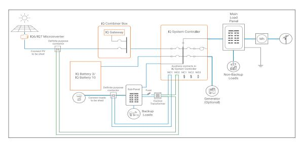
Line diagram for auxiliary contact connections used for shedding excess load and PV.
