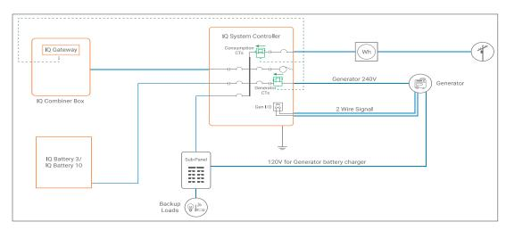
Line diagram for 2-wire remote start generator connection
