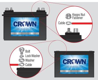
The battery terminal surface should be clean and dry prior to installation and torquing of the connectors to the terminals. Never place a washer or terminal treatment material between the battery terminal surface and the connector surface as this will increase electrical resistance - which affects battery and charger performance and can create potential safety hazards.
