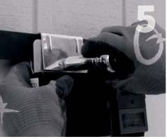
Tighten the cap screw with a half-inch socket and torque wrench to a torque of 15 foot-pounds.
