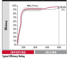
Real world efficiency with variable loads GS8048A: 93% CEC Efficiency Rating Most stringent US rating GS8048A: 92.5%
