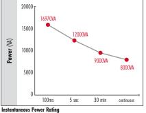
Instantaneous Power Rating Most stringent, massive load start 6S8048A: 16970VA Surge Power Rating Less stringent load start 6S8048A: 12000VA Peak Power Rating Frequent "heavy duty" load requirements 6S8048A: 9000VA Continuous Power Rating Sustained "real world" load requirements 6S8048A: 8000VA
