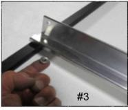
**For T-Slot Rails**: Lay T-Slot rails across the short axis of the panel as shown in Photo #1. Slide stainless bolts into T-slot of rail and position so they are opposite to the mounting holes on the
