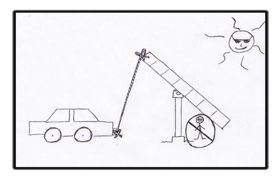
**DO NOT** stand between post and lower side of the array while seasonally adjusting tilt angle.
