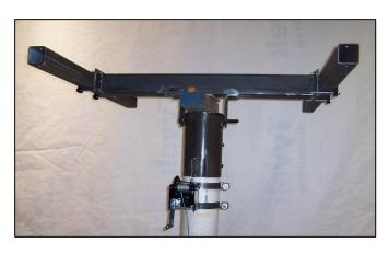
Install 2 cross pieces. Make sure small socket head bolts reference either side of center tube end plates. Leave 5/8" x 6" clamp bolts just slightly less than tight to facilitate installing longitudinals in next step.
