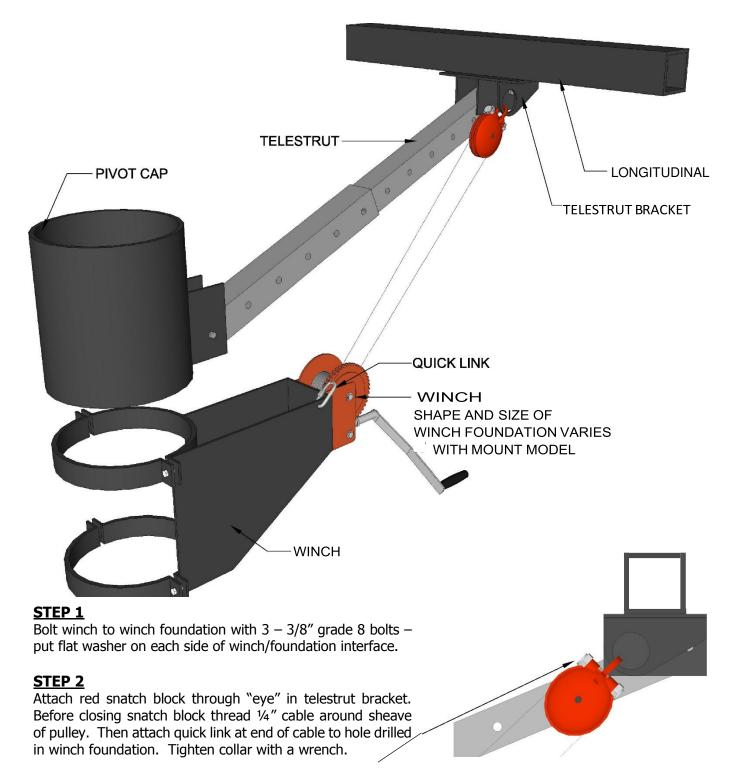
Be sure to thread nylon nut on closure bolt for snatch block all the way down to end of threads.
