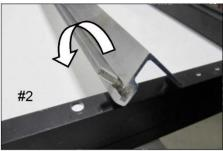
Lay T-Slot rails across the short axis of the panel as shown in Photo #1. Slide stainless bolts into T-slot of rail and position so they are opposite to the mounting holes on the frame of the panel as shown in Photo #2.
