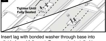
Insert lag with bonded washer through base into pilot hole and fully seat. Base can be installed in either orientation shown. Seal or flash base as needed. If deck level flashing is required, approved flashing methods include user-supplied, adhesive-backed, flexible flashing.
