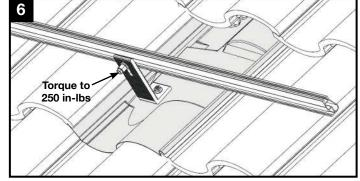
Attach rail to either side of L-Foot with bonding hardware. Ensure L-Foot does not extend above rail. Torque hardware to 250 in-lbs (21 ft-lbs).
