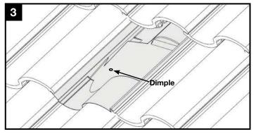
Insert Tile Replacement Flashing, lower onto base and apply pressure over the threaded post until it dimples the flashing.
