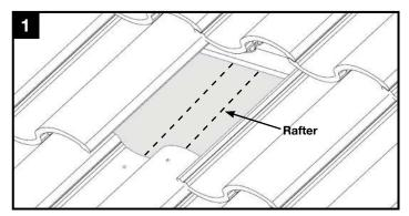
Remove tile and mark rafter. Use base as guide to drill 1/4" pilot hole and fill with roofing manufacturer's approved sealant.
