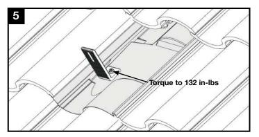
Form flashing as needed to sit flush with surrounding tiles. Position L-Foot in desired orientation and torque hardware to 132 in-lbs (11 ft-lbs).
