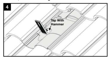
Place L-Foot over top of dimple and tap with hammer to punch the threaded posted through the flashing. Ensure punched pieces of flashing are cleared away.
