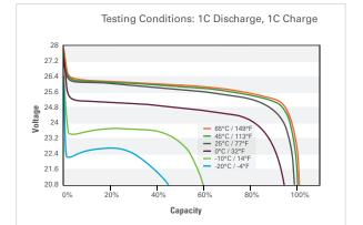
**DISCHARGE VOLTAGE IN RELATION TO THE TEMPERATURE**
