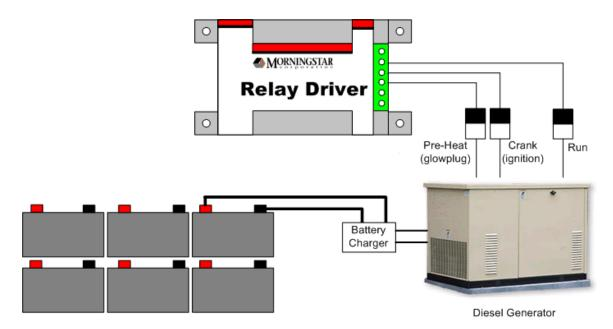
The first set up is the generator start and stop. In stand alone mode, the Relay Driver accomplishes this with battery voltage readings (taken at its own power terminals) as shown in Fig 6.
