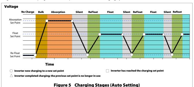
Figure 5 shows the progression of steps of the **Auto** charging cycle.
