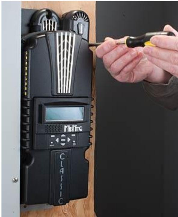
12. Holding the front cover with one hand, place a screw in the top left hole of the front cover and screw it into the top right hole of the back casting.
