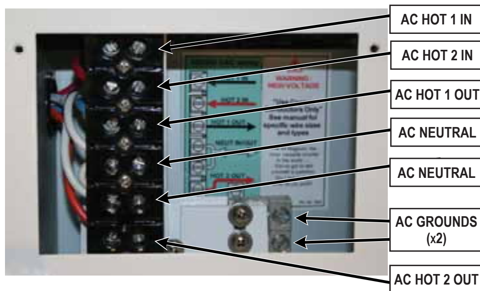
Figure 2-12, AC Terminal Block
