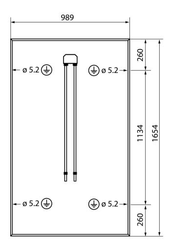
Figure 2: Module drawing
