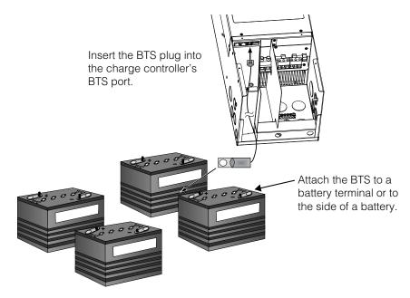
Figure 2-15 Installing the BTS
