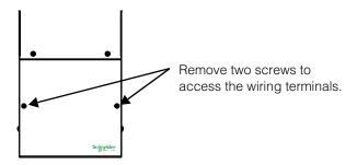
Figure 2-2 Removing the Wiring Compartment Cover
