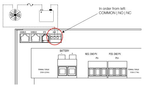
Figure 2-11 Auxiliary Output Vent Fan Application
