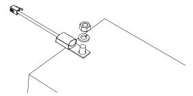
Figure 2-14 Attaching the BTS to a battery terminal
