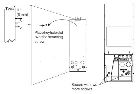
Figure 2-6 Mounting the Charge Controller
