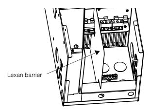
Figure 2-3 Wiring Compartment with Lexan Barrier
