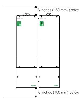
Figure 2-1 Minimum Clearance Requirements
