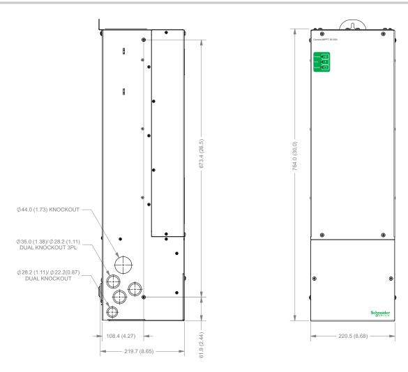
Figure 2-5 Dimensions and Knockout Locations
