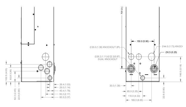
Figure 2-4 Knockout Dimensions
