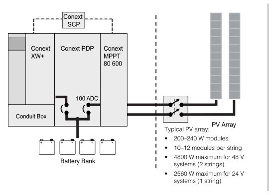
Figure 1-1 Typical Installation
