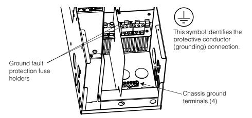
Figure 2-7 Chassis ground connector
