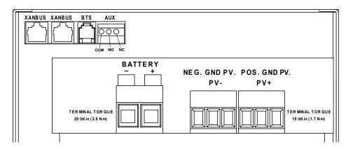
Figure 2-8 DC Terminal Connector Locations
