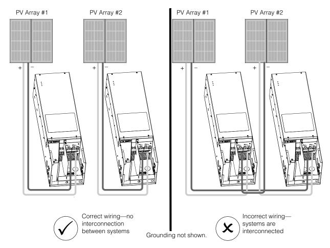
Figure 2-10 Multiple Unit DC Wiring
