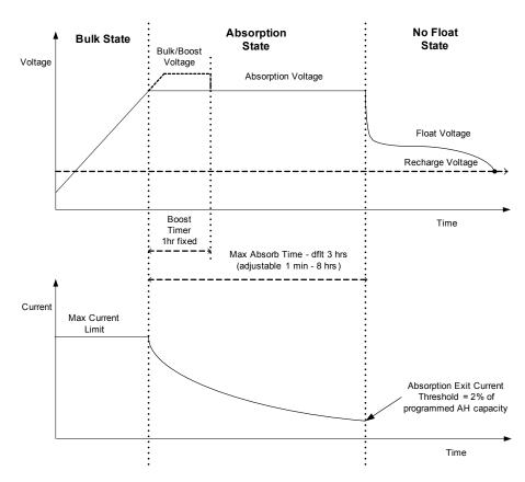
Figure 1-3 Two-stage Battery Charging Cycle
