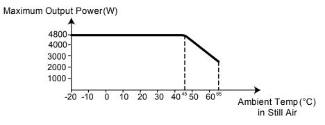
Figure A-4 Output power vs. ambient temperature
