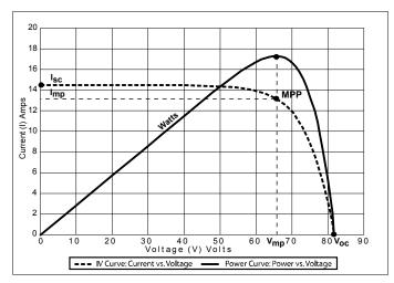
Figure 1-1 Maximum Power Point Curve
