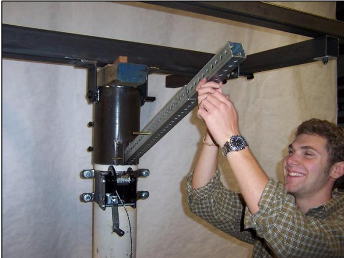
Install the 2 1/4" x 2 1/4" end of telestrut between the lugs on the bottom of the pivot cap. Tighten the nyloc nut all the way.
