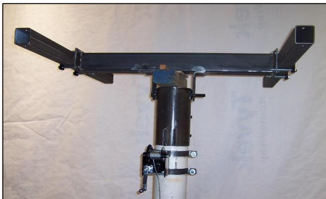
Install 2 cross pieces. Make sure small socket head bolts reference either side of center tube end plates. Leave 5/8" x 6" clamp bolts just slightly less than tight to facilitate installing longitudinals in next step.
