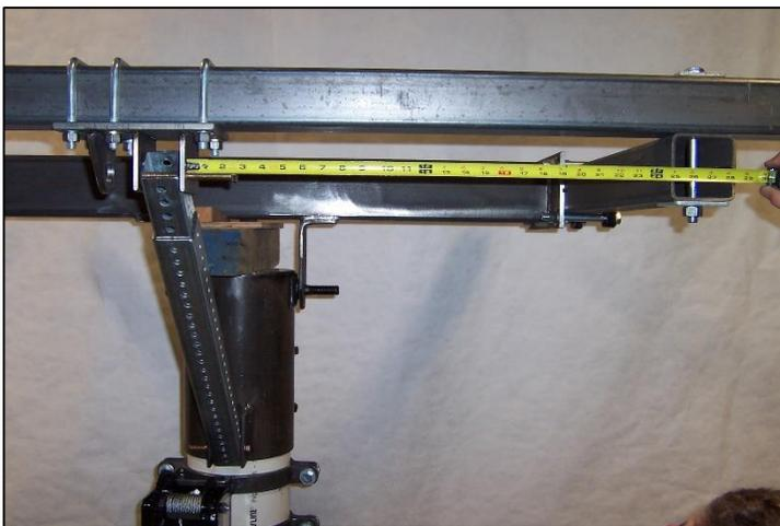
Insert 7/16" bolt through lugs and upper end of telestrut and tighten. Make sure middle bolt is installed through telestrut in the hole that is circled, tighten nyloc onto bolt.
