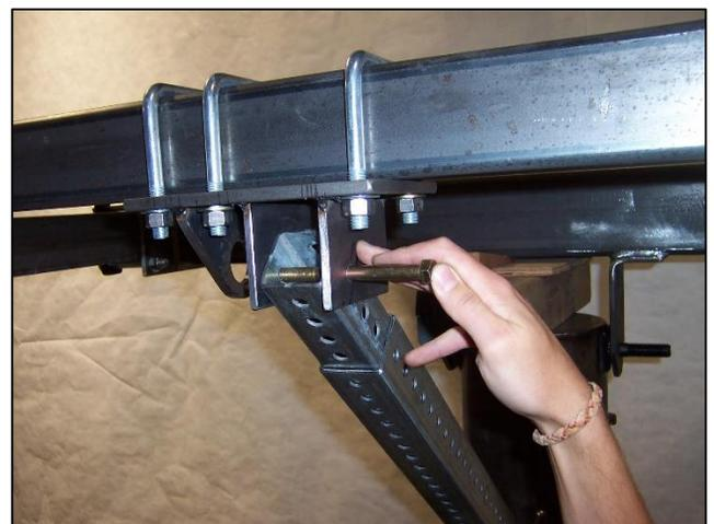
Attach orange pulley to pad eye on telestrut bracket. Thread cable with quick link connector through pulley before closing pulley hanger with 3/8" bolt and nyloc nut. Now attach quick link to hole on left side of winch foundation (see attached Winch Detail).
