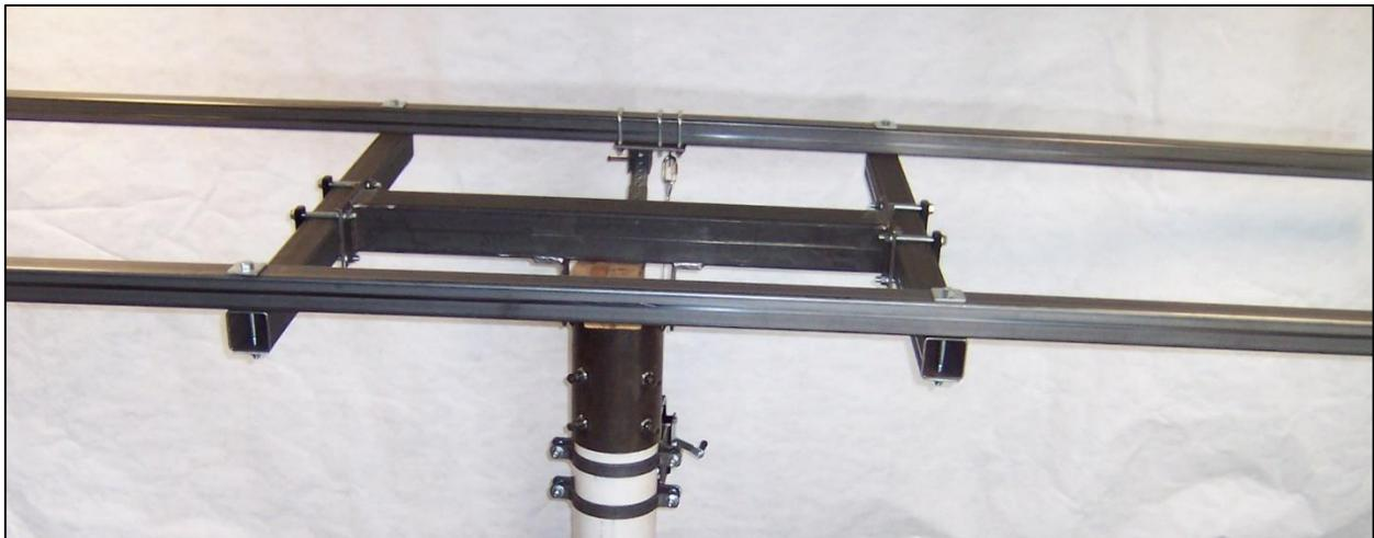
Move the longitudinals as close as possible to horizontal to one another to begin installing rails. 15X and 18X use channel rails and have no brackets. 12XHD uses angle rails and brackets to attach rails to the longitudinals.
