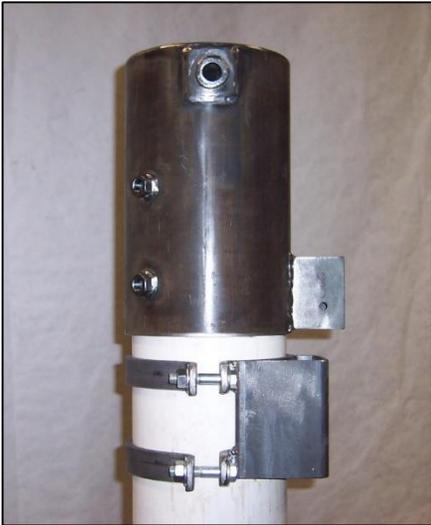
Place pivot cap on top of steel post. Orient pivot bore with bronze bushings east and west. The 4 set bolt nuts should face south. Secure the pivot cap with  $\frac{3}{4}$ " square head set bolts.
