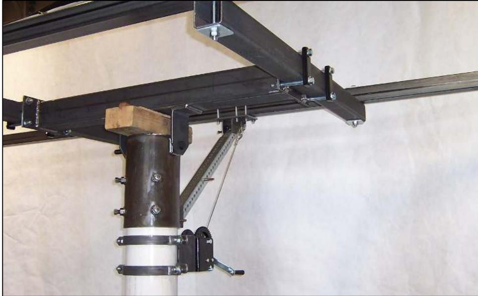
Wind up all the slack. Then it is safe to remove wedges and wood block.
