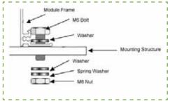
*Figure 2. Securing the module with bolts.*
