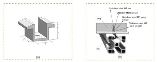
Figure 5. Close-ups of middle (a) and side (b) aluminum clamps. The dimensions for the middle clamps are  $a \ge 40$  mm,  $b \ge 26$  mm, c = 8 mm,  $d \ge 28$  mm, and  $\emptyset = 9$  mm.
