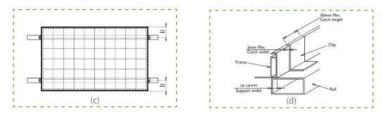
Figure 3. Illustrations of the three different methods for clamping modules onto the frame with aluminum clamps.
