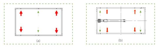
Figure 1. Bolt positions for the at-minimum four-bolts for a) modules CHSM5409M, CHSM6609M/P, CHSM6610M/P; and b) modules CHSM6611P and CHSM6612P. Solid red arrows indicate primary bolt positions; dashed blue arrows indicate positions where bolts can be added for additional support.
