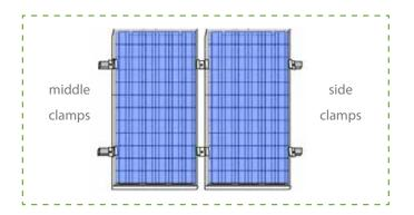
Figure 4. Placement of middle and side clamps on the modules
