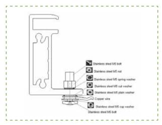
Figure 7. Grounding the aluminum frame with copper wire.
