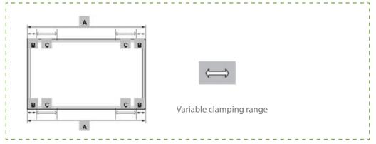
Figure 6. Permitted clamping locations with clamp. For exact dimensions for a given module series, see table 1 (below).
