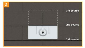
Slide flashing, between 1st and 2nd course, so the top is at least 3/4" above the edge of the 3rd course and the bottom is above the edge of the 1st course.
