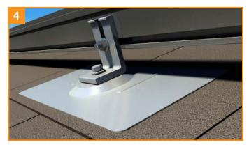
The FlashFoot is now installed and ready for IronRidge Rails. With provided L-foot fasteners preloaded into rails, drop rails into open L-foot slots.
