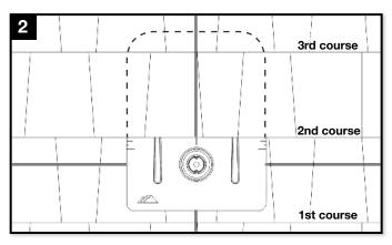
Slide flashing, between 1st and 2nd course, so the top is at least 3/4" above the edge of the 3rd course and the bottom is above the edge of the 1st course.
