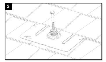
Line up pilot hole with flashing hole and insert lag bolt with bonded washer through flashing. Tighten lag bolt until fully seated.
