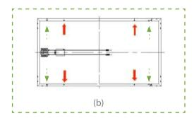
Remark: As for above diagram, the solid red arrows indicate primary bolt positions; dashed blue arrows indicate positions where bolts can be added for additional support.
