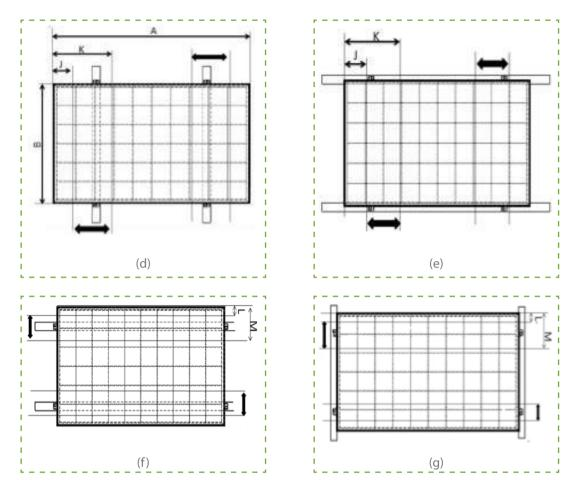
Remark: Illustrations (figure d、e、f、g) of the four different methods for clamping modules on the frame with aluminum clamps. "means the aluminum clamp's permissible clamping range. The recommended installation position shows as below table:
