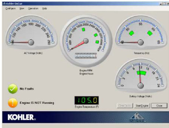
OnCue User Interface Screen (ADC 2100 version shown)
