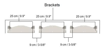
Figure 18: Brackets spacing
