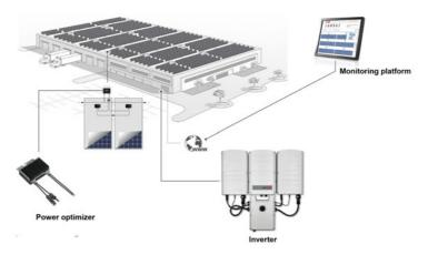
Figure 1: The SolarEdge power harvesting system components
