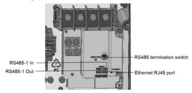
Figure 33: Connection Unit Communication board
