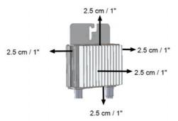
Figure 4: Power optimizer clearance
