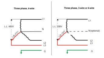
Figure 3: AC grids supported by SolarEdge three-phase inverters
