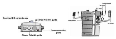
Figure 13: Connection Unit bottom and side interface
