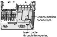
Figure 39: Inserting communication cables
