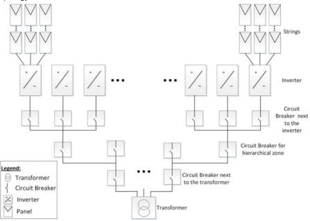
Figure 52: Typical transformer and commercial three phase inverter installation topology
