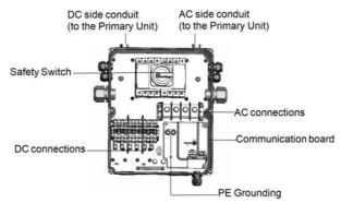
Figure 26: Inside the Connection Unit
