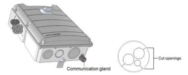
Figure 35: Communication gland and rubber fitting
