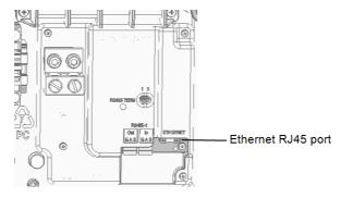
Figure 38: Connection Unit Communication board
