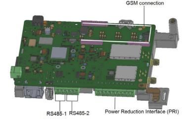
Figure 32: Primary Unit communication board
