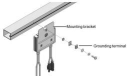
Figure 7: Power optimizer grounding terminal
