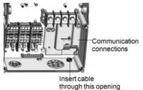
Figure 37: Inserting communication cables
