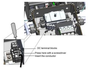
Figure 25: Connecting the DC wires
