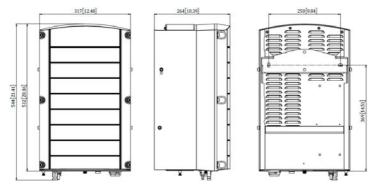
Figure 46: Secondary Unit - front, side and rear views
