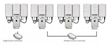
Figure 34: Example of Ethernet connection
