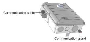
Figure 31: Connection Unit bottom
