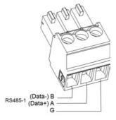
Figure 41: RS485 terminal block wire connections
