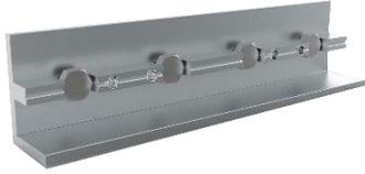
1/4" Slot Open Rail Splice Kit with 4X 1/4-20 Bolts and Flange Nuts with integral grounding. **May be repositioned until torqued to final value.**
