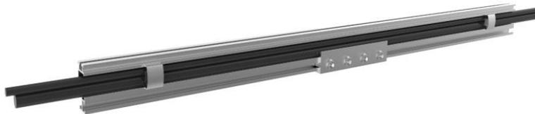
The HR150 family of products are shown assembled above. Two HR150 Rails are spliced together with an HR150 Rail Splice. PV electrical wires are shown routed in the channels of the HR150 Rails, retained with two HR150 Channel Clips snapped into place.
