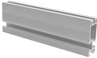
Helio Rails: Features both 1/4" and 3/8" side slots, and 1/4" top slot for clamping PV panels. Available in 84", 124", 164" and 206" lengths. Last 3 digits denote rail length. 4 stock sizes in clear and black.
