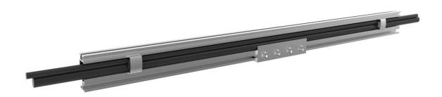
The HR150 family of products are shown assembled above. Two HR150 Rails are spliced together with an HR150 Rail Splice. PV electrical wires are shown routed in the channels of the HR150 Rails, retained with two Wire Covers snapped into place.
