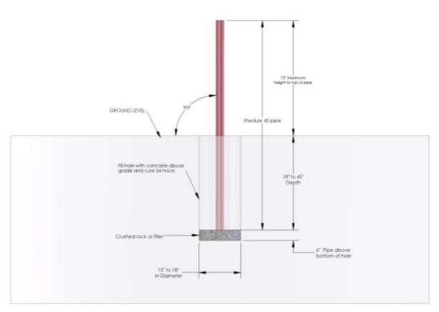
Figure 1 Side of Pole Foundation Guideline Diagram
