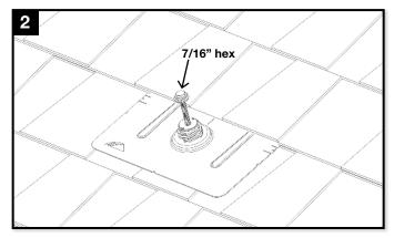
Fill hole in dock with roofing manufacturer's approved sealant. Insert screw with bonded washer through hole. Tighten screw until fully seated.
