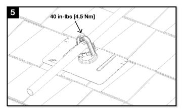
Adjust top bolt so saddle is snug on the conduit. Tighten bolt on top of saddle to 40 in-lb [4.5 Nm].
