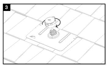
Place Conduit Cap on dock and rotate 180 degrees to secure.
