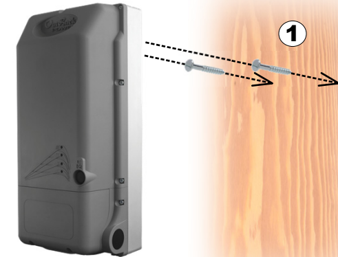
Keyhole Slots (#14 slotted wood screws, 7.9" or 20.1 cm spacing)
