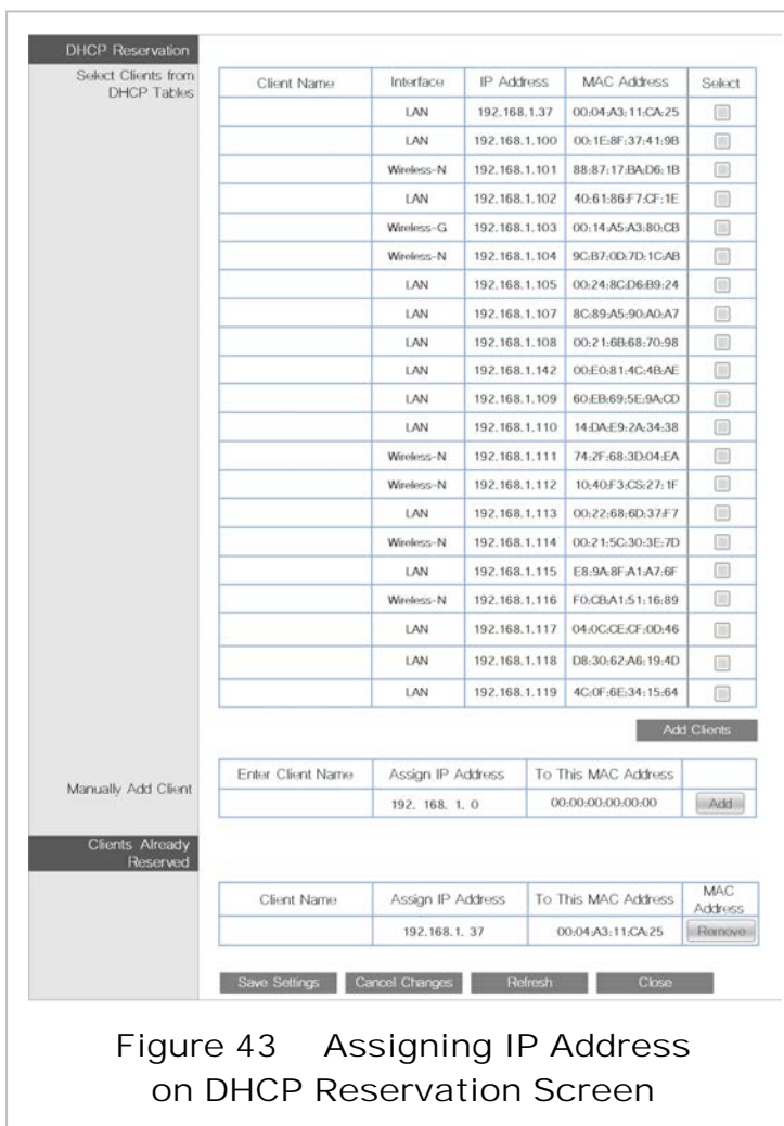
Figure 42 DHCP Reservation on Cisco Router
