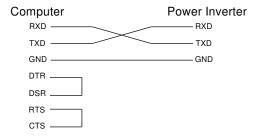
6-1-3. The RS-232 interface of this unit employs ASCII code to implement the asynchronous serial transmission control.
