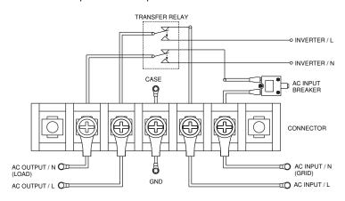
• Connect AC input wiring to the inverter socket.
