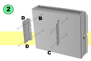
Place the rear brackets on the BOS studs (**B**). Attach the rear brackets to the BOS assembly using the four M6 nuts provided (**C**). Ensure that the pegs on each bracket (**D**) face inward (toward the opposite bracket).
