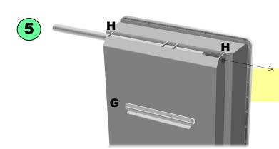
Install the SkyBox onto the wall bracket by lifting it into position. The SkyBox is equipped with rear brackets which are already attached (**G**).
