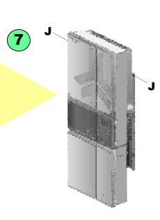
The wall bracket has securing holes for the SkyBox (**J**). Secure the SkyBox in place by inserting an M6 × 40 mm screw on each side.
