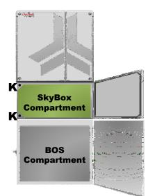
Two areas house the system wiring. The BOS compartment opens with a latch. It connects to external wiring (battery, AC, PV, etc.) and conduit. These connections extend from the BOS into the SkyBox compartment, which opens with two Allen screws (**K**). If the SkyBox must be removed for service, the BOS and its wiring can remain. Some connections, such as communications, pass through the BOS to be made directly in the SkyBox.
