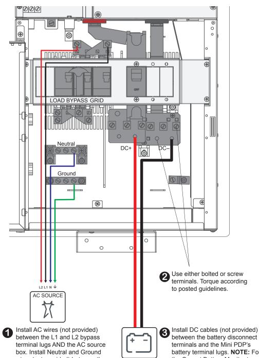
Install AC wires (not provided) between the L1 and L2 bypass terminal lugs AND the AC source box. Install Neutral and Ground wires (not provided) between the Neutral and Ground bus bars AND the AC source box. Route the wires through one of the knockout holes.
