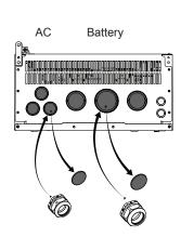
Remove the DC knockout plugs and set aside.
