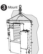
Fasten backplate screws (3/8 in screws, not supplied)
