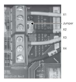
Secondary transformer wire X1, X2, X3, and X4 locations AFTER reconfiguration
