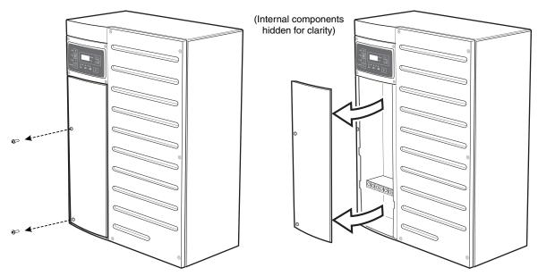
Figure 3-1 AC access panel removal
