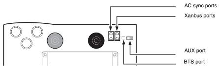
Figure 3-3 Conext XW+ Inverter/Charger communication ports
