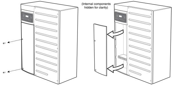
Figure C-2 AC access panel removal
