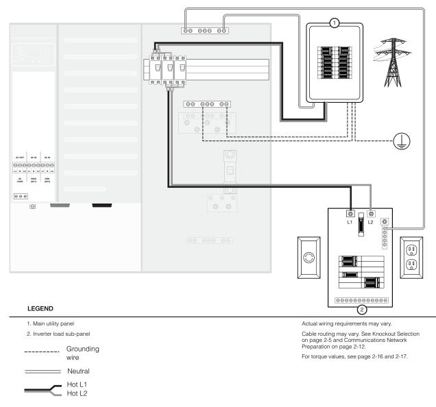
Figure 3-15 Wiring the PDP to the Inverter Load Sub-Panel or Utility Grid
