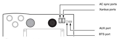
Figure 4-4 Conext XW+ Inverter/Charger communication ports
