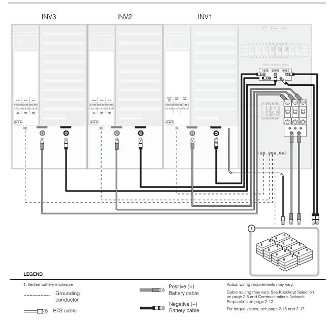
Figure 3-27 DC Connections for a Triple-Inverter System
