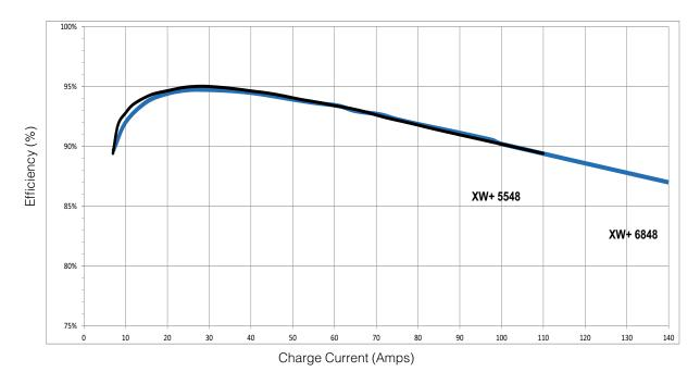
Figure A-4 Charging Efficiency (Typical)
