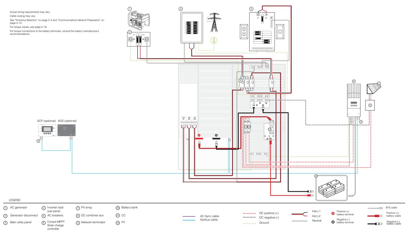
Figure B-3 Single-Inverter System Renewable Energy (Solar)
