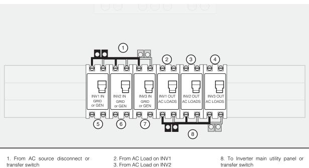
transfer switch NOTE: Install L1 power distribution bar (jumper) in first GRID/GEN breaker slot facing FRONT. From AC Load on INV I
