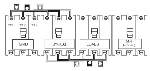
Figure 3-32 Power Distribution Jumper Installation (Three-Phase)
