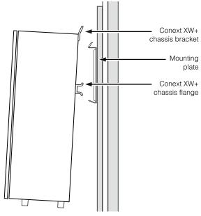
Figure 2-7 Wall-mounting the Conext XW+
