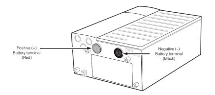
Figure 3-7 Battery terminals (bottom of Conext XW+)
