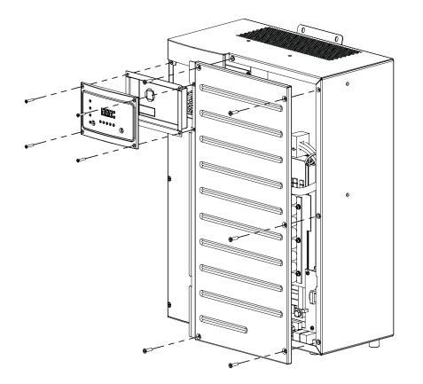
5. For easier access, remove the right-side panel of the Conext XW+, as shown in Figure 5-3.
