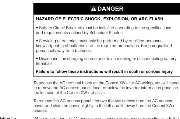
**Installation tip** When re-securing the AC access cover, ensure its recessed edge slips inside the edge of the front panel.
