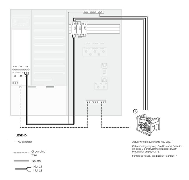
Figure 3-14 Wiring the PDP to a Generator (Off Grid)
