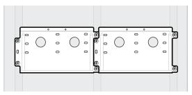
Figure 2-6 Two interlocking mounting plates
