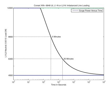
Figure A-1 Conext XW+ AC Overload Capability
