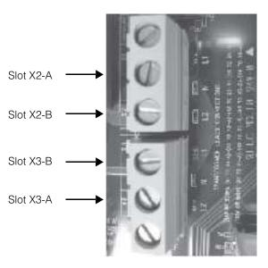
Figure C-4 Slot Locations on X1 and X2 Connectors
