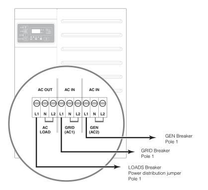
Figure 3-34 Inverter/Charger Three-Phase AC Wiring
