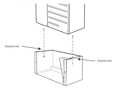
Figure 2-8 Conduit Box keyhole alignment
