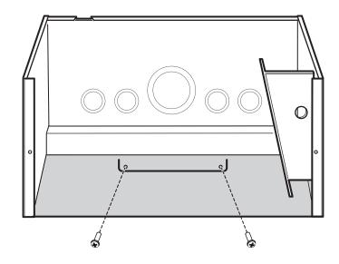
Figure 2-9 Wall-mounting the Conduit Box
