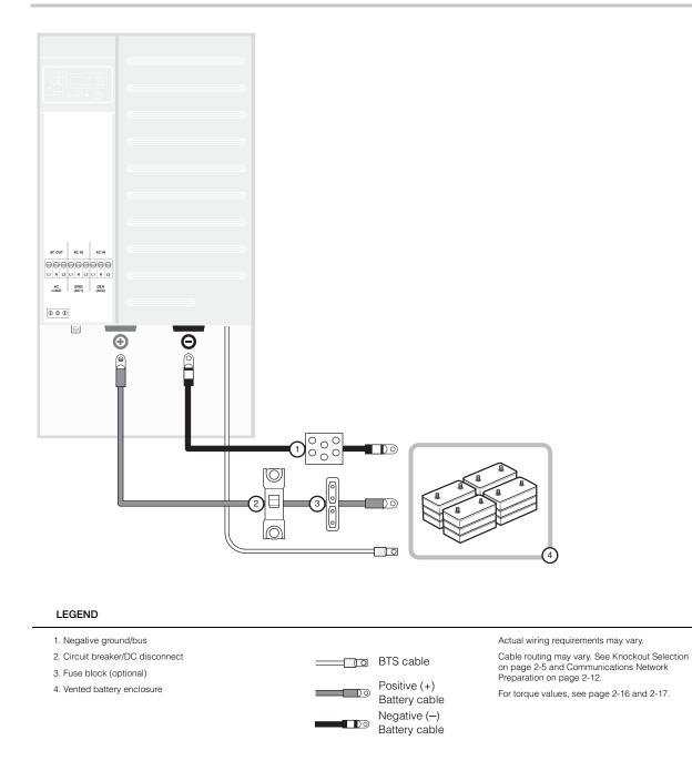
Figure 3-37 DC Connections to a Single Inverter (No PDP)
