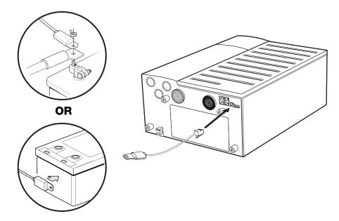
Figure 3-6 Battery Temperature Sensor Installation
