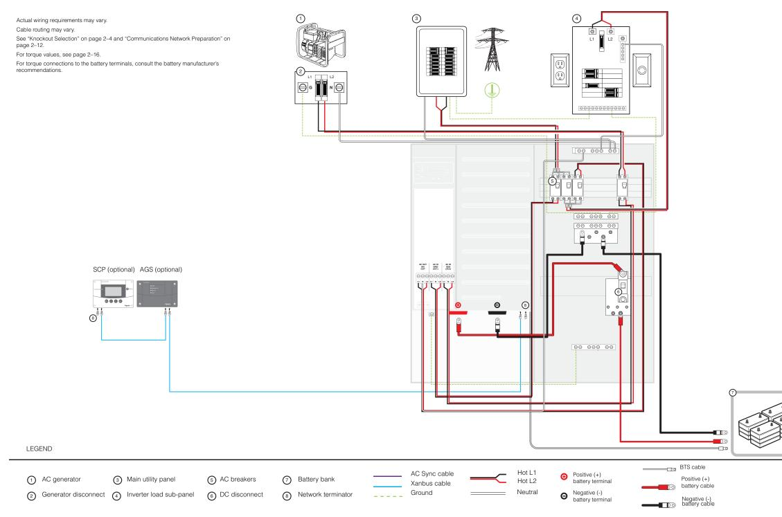
Figure B-2 Single-Inverter System (Backup Only) With a Conext XW+ Power Distribution Panel
