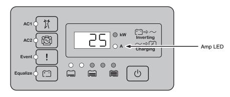
Figure 3-21 Checking Charging Operation
