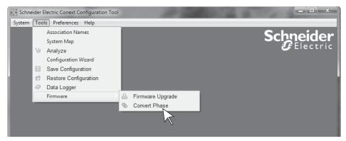
Figure C-7 Upgrading the firmware
