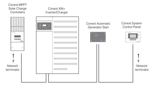
Figure 4-1 Xanbus Network System (Example)
