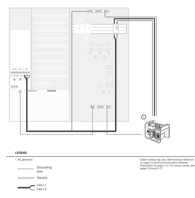
Figure 3-13 Wiring the Conext XW+ Power Distribution Panel to a Generator (On-Grid)
