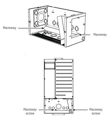
Figure 4-5 XW+ Conduit Box raceways
