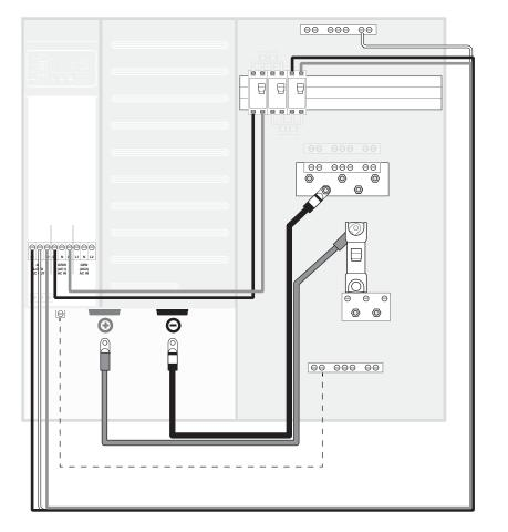
Wiring the Conext XW+ Inverter/Charger with a PDP
