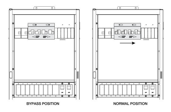
Figure 3-26 Installing the custom designed bypass interlock plate
