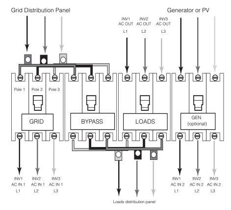
Figure 3-33 PDP Three-Phase AC Wiring
