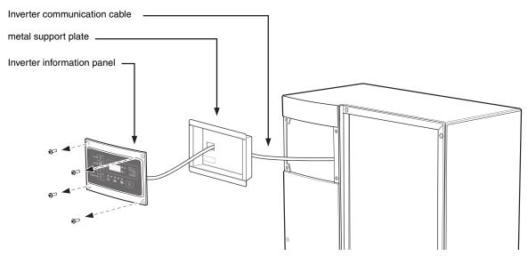
Figure 5-2 Inverter information panel removal
