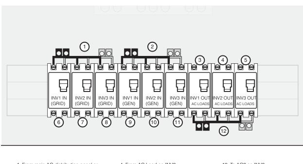
1. From main AC distribution panel or transfer switch NOTE: Install L1 power distribution bar (jumper) in first GRID/GEN beaker slot facing FRONT.
