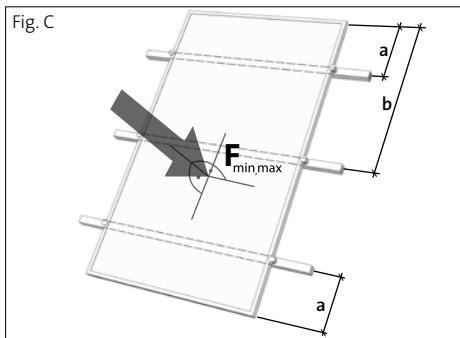
**a** = 223 mm (8.8 in)\*       $F_{\min} = -3,4 \text{ kN/m}^2$  (- 76 psf)
