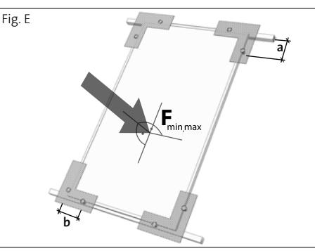
**a** = 239 mm (9.4 in)       $F_{\min} = -1,44 \text{ kN/m}^2$  (- 30 psf)
