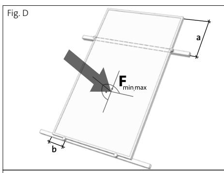
**a** = 510 mm (20.1 in)\*       $F_{\min} = -2,4 \text{ kN/m}^2$  (- 50 psf)
