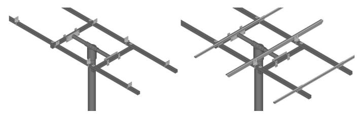
Attach aluminum angle brackets to longitudinals with smaller square U-Bolts and whiz flange nuts. Oppose aluminum angle brackets as shown. Some mounts come with aluminum angle rails with punched holes for bolting on panels, and some come with aluminum extrusions which allow for panel attachment bolts or clips to slide in the "t-slot".
