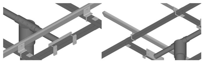
Attach aluminum rails as shown. If rail ends are marked "TOP", align them to the same end.
