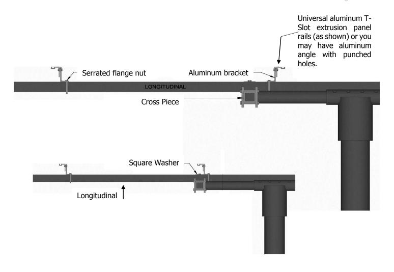
Bracket orientation in most installations is generally opposed to one another as in top picture. It may be necessary to have brackets facing in same direction as in bottom picture, if panel size is such that you need to do this to maintain a 1/4" gap between panel ends on centerline.
