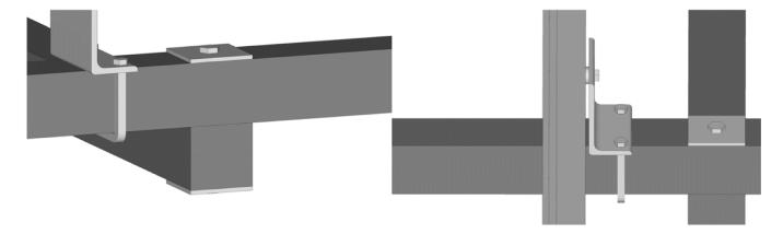
**General view of assembly**. When fastening panels to rails, place first panels at end of rails marked "TOP" and work down until all panels are in place with bolts finger tight. Cross measure array for square, check to see that all spaces (approx. 1/4") between panels are equal, then tighten all bolts.
