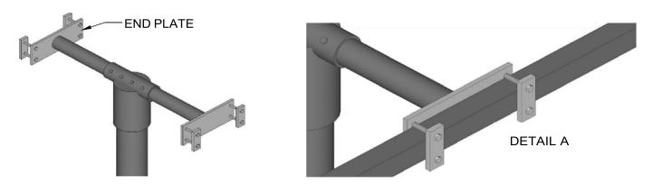
Finger tighten onto "Tee" end plates, aluminum flat bar and straight 1/2" bolts. Place entire "Tee" assembly on top of post. The aluminum flat bar and straight 1/2" bolts are shown in Detail "A".
