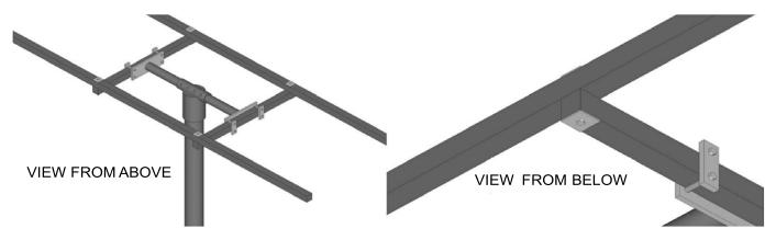
Place longitudinal tubes on top of cross pieces and bolt with square washers top and bottom.
