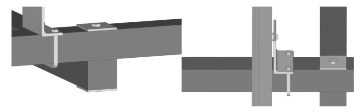
**General view of assembly**. When fastening panels to rails, place first panels at end of rails marked "TOP" and work down until all panels are in place with bolts finger tight. Cross measure array for square, check to see that all spaces (approx. ¼") between panels are equal, then tighten all bolts.
