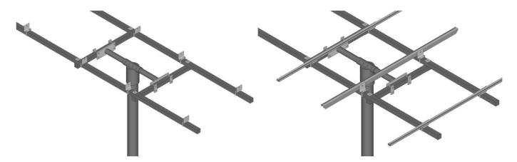
Attach aluminum angle brackets to longitudinals with smaller square U-Bolts and whiz flange nuts. Oppose aluminum angle brackets as shown. Some mounts come with aluminum angle with punched holes for bolting on panels, and some come with aluminum extrusions which allow for panel attachment bolts or clips to slide in the "t-slot".
