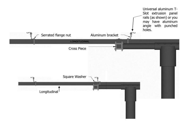
Bracket orientation in most installations is generally opposed to one another as in top picture. It may be necessary to have brackets facing in same direction as in bottom picture, if panel size is such that you need to do this to maintain a ¼" gap between panel ends on centerline.
