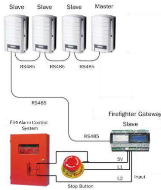
Figure 7: Example: Emergency Stop Button and Fire Alarm System Connection
