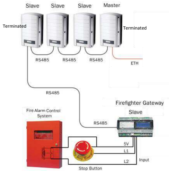
Figure 10: Example of RS485 Connection
