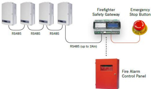
Figure 2: The SolarEdge Firefighter Gateway Connections
