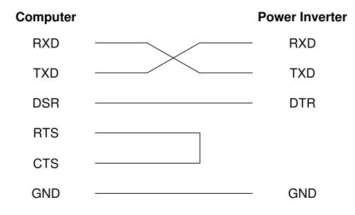
8-1-3. The RS232 interface of this unit employs ASCII code to implement the asynchronous serial transmission control. The byte structure is START BIP – 8 BIT DATA-STOP BIT Baud rate : 1200,2400,4800,(SET BY DIP-SW).
