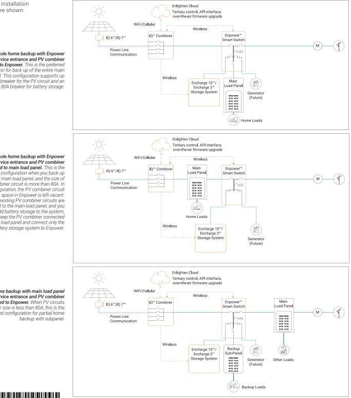
Whole home backup with Enpower as service entrance and PV combiner connected to Enpower. This is the preferred configuration for back up of the entire main load panel. This configuration supports up to an 80A breaker for the PV circuit and an
