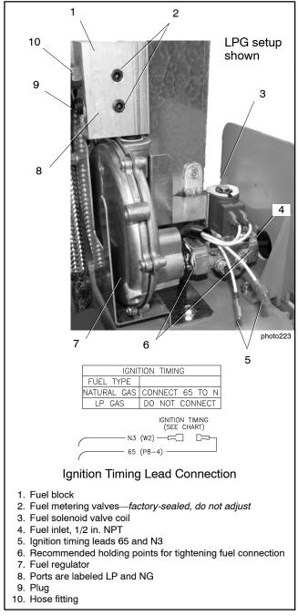
Figure 1-9 Fuel System, 14RESA/RESAL Equipped with Fuel Block (built before June 26, 2014)
