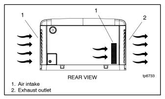
Figure 1-3 Cooling Air Intake and Exhaust
