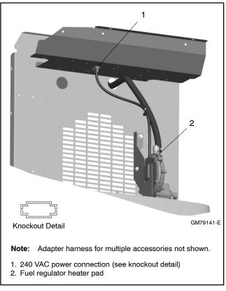
Figure 2-6 Model 20RESA/RESAL/RESC/RESCL 240 Volt Kit Power Connection
