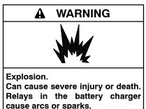
Locate the battery in a well-ventilated area. Isolate the battery charger from explosive fumes.
