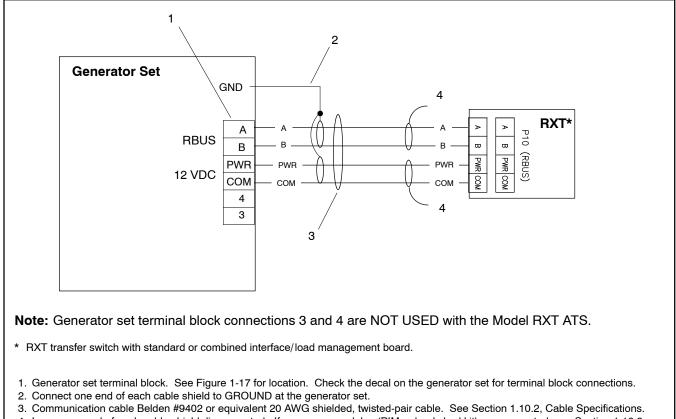
4. Leave one end of each cable shield disconnected. If accessory modules (PIM or load shed kit) are connected, see Section 1.10.3.
