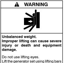
Lift the generator set using lifting bars inserted through the lifting holes on the skid.
