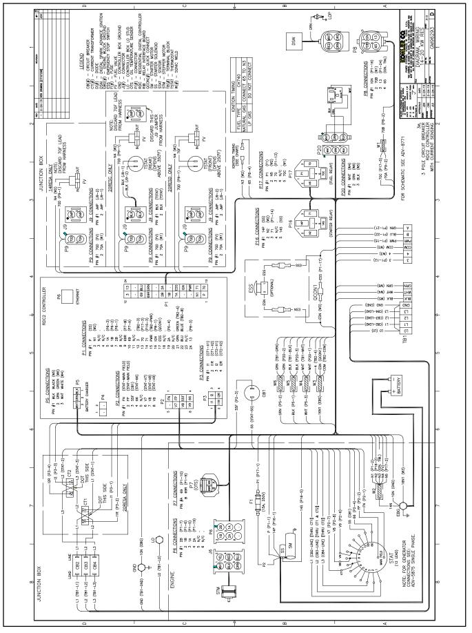
Figure 3-22 Wiring Diagram, Model 20RESC/20RESCL, GM96293, Sheet 3 of 3
