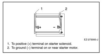
Figure 1-29 Typical Battery Connection
