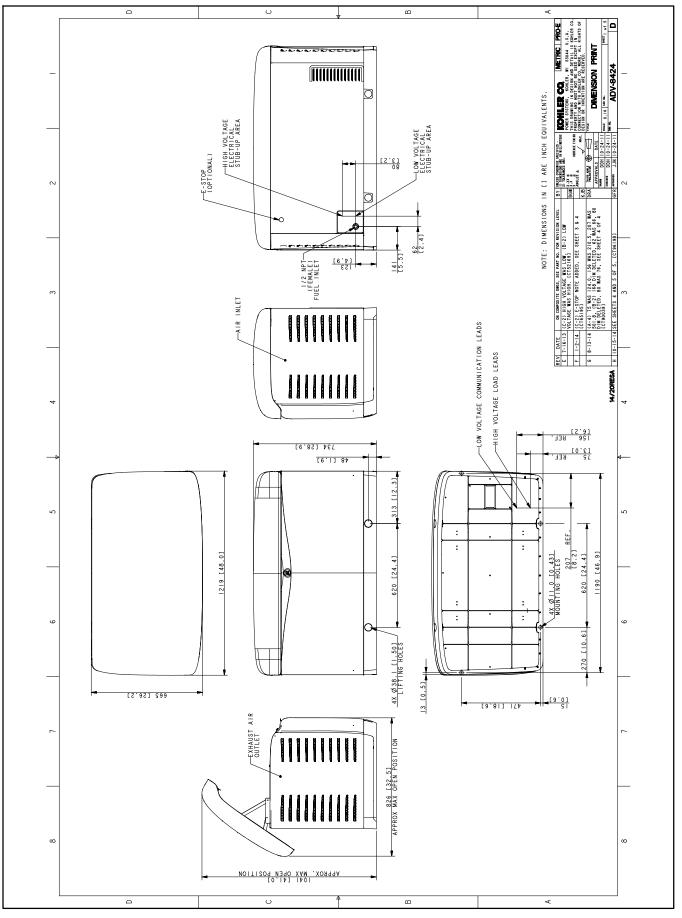
Figure 3-2 Dimension Drawing, 14/20RESA/RESAL, ADV-8424, Sheet 1 of 5
