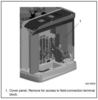
Figure 1-17 Field-Connection Terminal Block Location
