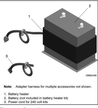
Figure 2-14 Battery Heater
