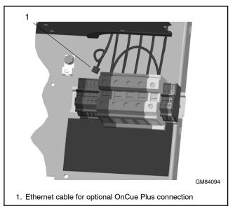
Figure 2-16 Network Connection for OnCue Plus
