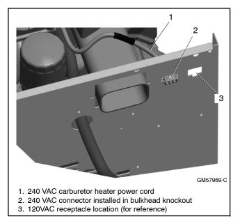
Figure 2-12 240 Volt Power Connection for Carburetor Heaters
