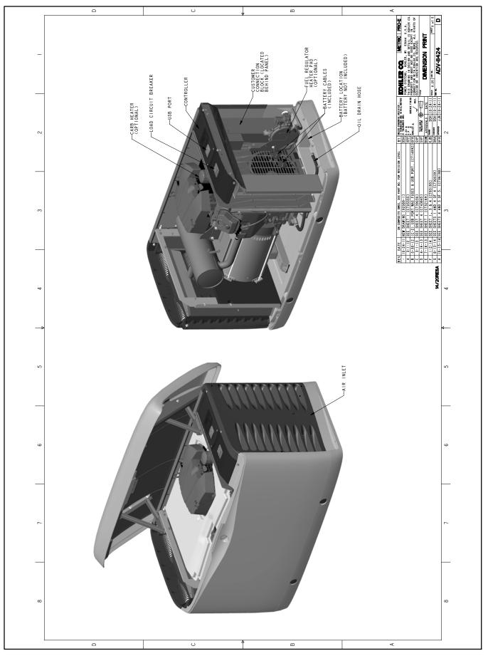
Figure 3-4 Dimension Drawing, 14/20RESA/RESAL, ADV-8424, Sheet 3 of 5
