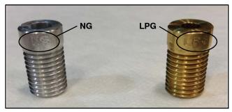
Figure 1-10 NG and LPG Fuel Orifice Fittings
