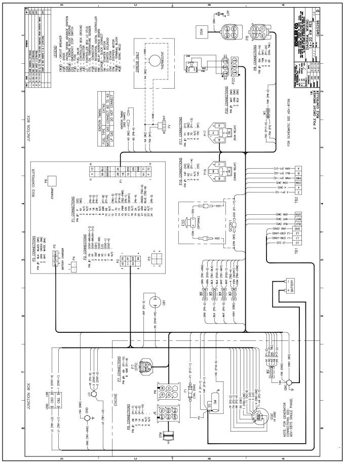
Figure 3-14 Point-to-Point Wiring Diagram, 14/20RESA/RESAL, GM93298, Sheet 1 of 3
