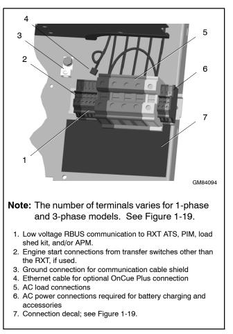
Figure 1-18 Field Connection Terminal Blocks
