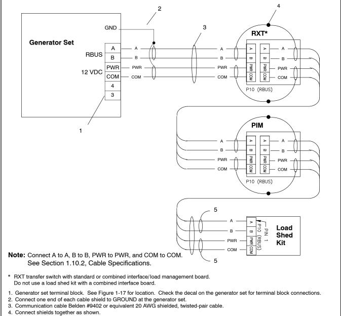
5. Leave one end of each cable shield disconnected at the last device.
