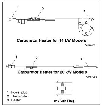
Figure 2-9 Carburetor Heaters
