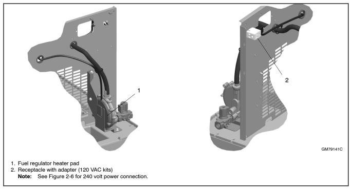
Figure 2-7 Installed Regulator Heater Kit (for 20RESA/RESAL/RESC/RESCL)
