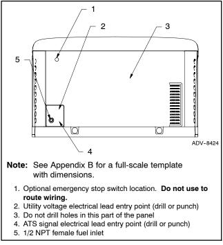
Figure 1-16 Electrical Lead Entry Locations
