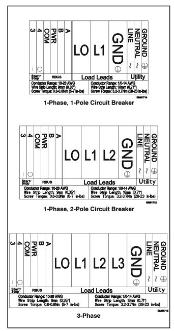
Figure 1-19 Terminal Block Connection Decals
