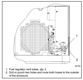
Figure 1-14 Fuel Regulator Vent Hoses
