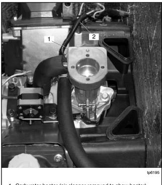
Carburetor heater (air cleaner removed to show heater)
