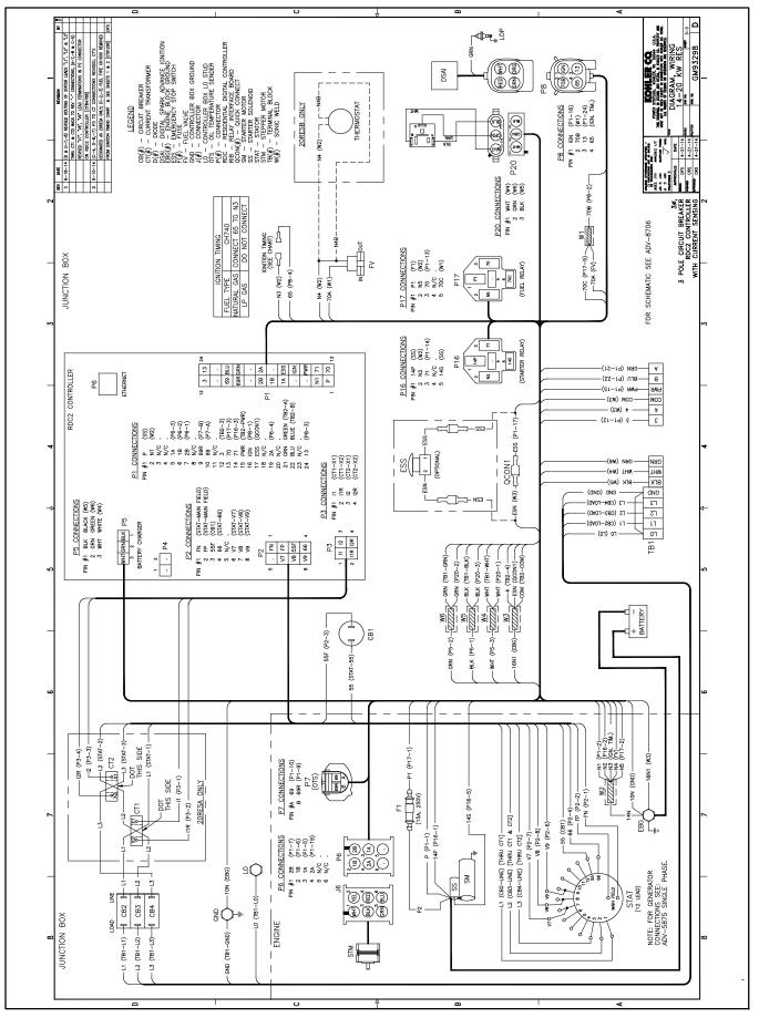
Figure 3-16 Point-to-Point Wiring Diagram, 14/20RESA/RESAL, GM93298, Sheet 3 of 3
