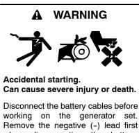
Remove the negative (-) lead first when disconnecting the battery. Reconnect the negative (-) lead last when reconnecting the battery.
