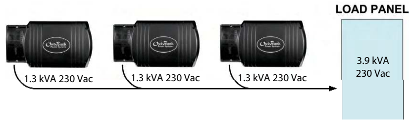
Figure 8 Example of Parallel Stacking Arrangement (Three Inverters)
