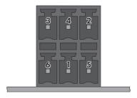
Figure 6: Pin assignment
