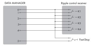
Figure 7: Connection of a Ripple Control Receiver
