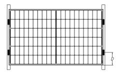
Fig. 9 Rails overlapping the short-side frame
