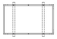
Fig 3. Bolt installation for 60cell
