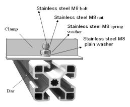
Fig. 12 Schematic diagram of the fringe clamp
