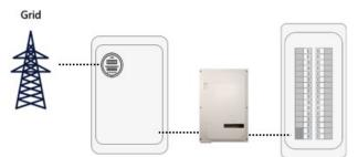
Partial home backup: Partial backup with a MSP that has an integrated meter offers backup capability with a reduced installation cost. This installation method will back up smaller loads, such as general lighting and receptacles, and leave larger loads such as HVAC, or dryers in the main panel. This method has lower installation costs and stored-energy longevity while in backup mode.
