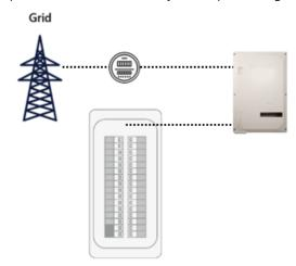
Whole home backup (combined meter and MSP): This method is comparable to a main panel upgrade and should be treated like one. There are two ways to connect the Backup Interface to the busing of the existing MSP. For either of these connection methods, the BI-Nxxxx (main lug only) variant is recommended.
