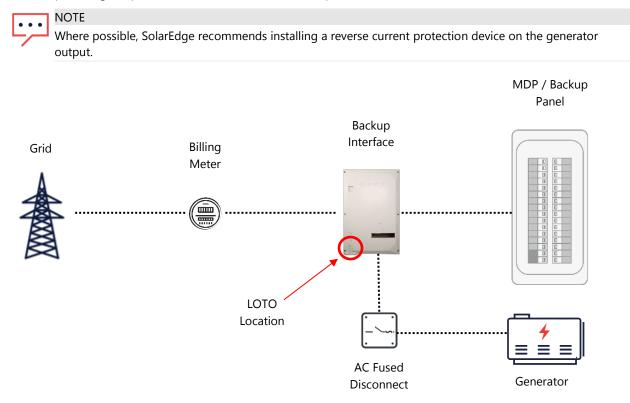
If the inverter is still on, it will go into backup mode, even if the main circuit breaker is locked into the open position. Install an emergency stop button to shut off the system. Refer to the installation manual for more details about the remote shutdown switch.
