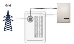
• Create an essential loads panel including all of the circuits from the main panel. The advantage of this method is safety, not having to work with the utility to isolate the MSP, and maintaining certifications and warranties of the existing equipment.
