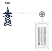
Meter main combination panel: This service entrance type is configured with the PCC and billing meter integrated into the MDP. This service entrance type is the most common in the continental US.
