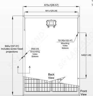
Dimensions in brackets are in inches. Un-bracketed dimensions are in millimeters. Unit: mm[in.]
