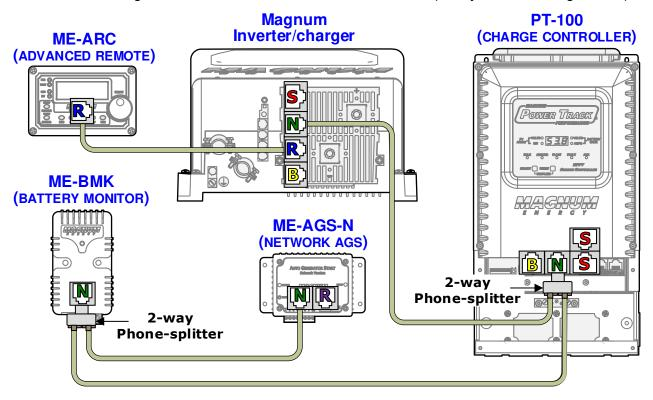
Note: The ME-AGS-N or PT-100 must be the first network device connected to the inverter, followed by the ME-BMK, and whatever device wasn't used as the first network device (ME-AGS-N or PT-100) is connected after the ME-BMK.
