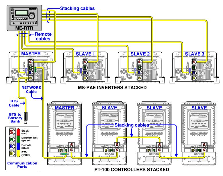
**CAUTION:** Do not network any PT-100 directly to the ME-RTR or damage may occur. Note: A phone-splitter can not be used in any configuration that has the ME-RTR installed.
