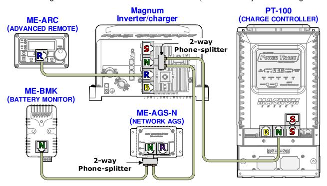
Note: The ME-AGS-N and PT-100 are the first network devices connected to the inverter, followed by the ME-BMK.
