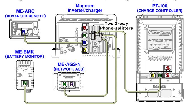
Networking the PT-100 with Other Network Devices (Star Configuration using a 3-way splitter)
