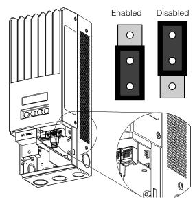
Figure 2-7 PV Negative Ground Jumper Location
