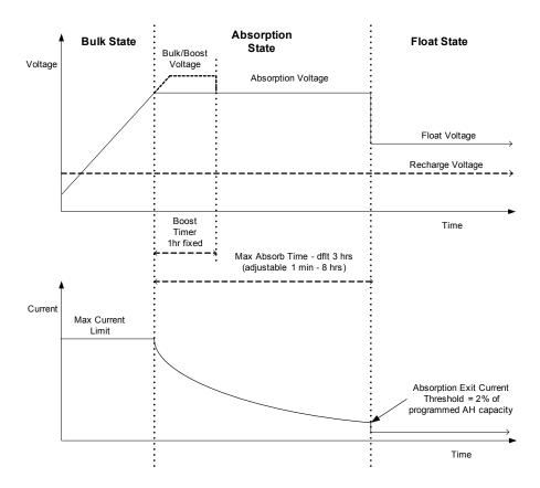
Figure 1-4 Three-stage Battery Charging Cycle<sup>a</sup>
