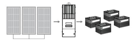
Figure 1-3 PV Charge Controller
