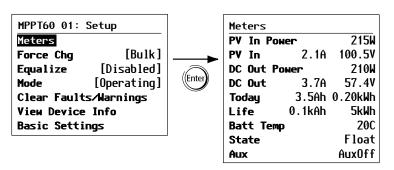
Figure B-9 Selecting the Meters Screen
