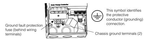
Figure 2-6 Charge Controller Safety Ground Connector
