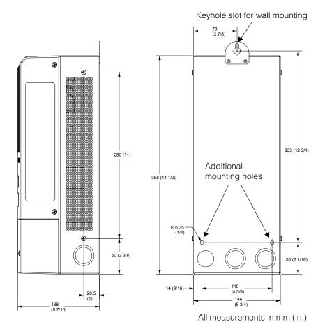
Figure 2-3 Dimensions and Knockout Locations
