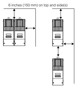
Figure 2-1 Minimum Clearance Requirements
