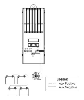
Figure 2-12 Auxiliary Output Vent Fan Application
