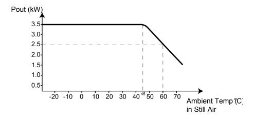
Figure A-1 Output Power vs. Ambient Temperature
