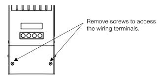
Figure 2-2 Removing the Wiring Compartment Cover
