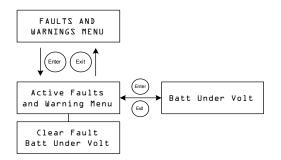
Figure 4-3 Faults and Warnings Menu
