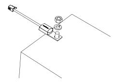
Figure 2-15 Attaching the BTS to a Battery Terminal
