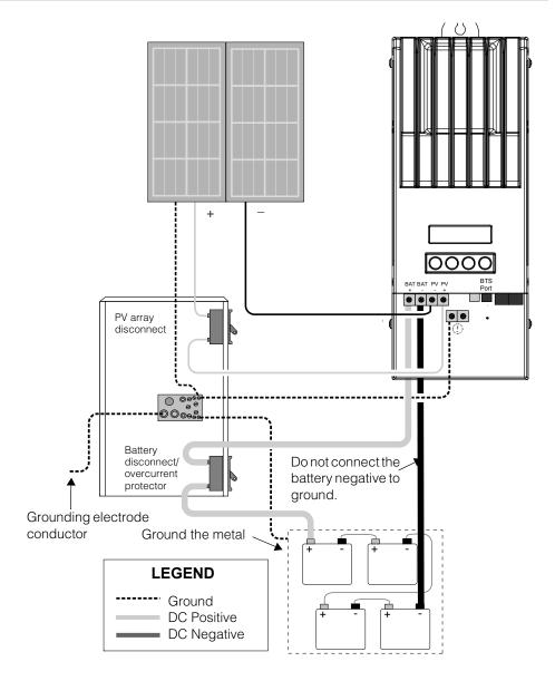
Figure 2-10 Charge Controller Power Wiring
