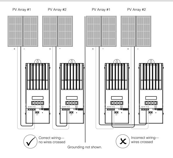
Figure 2-11 Multiple Charge Controller Array Wiring
