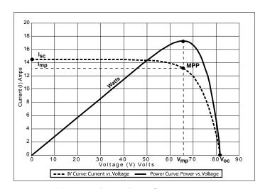
Figure 1-2 Maximum Power Point Curve
