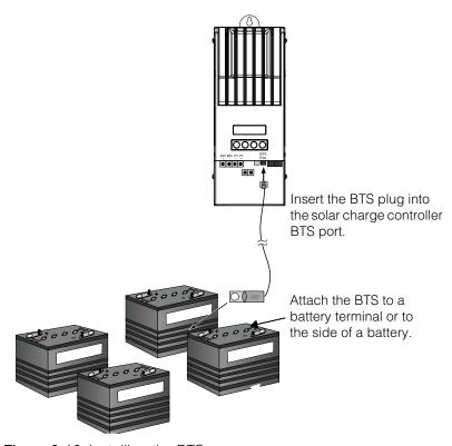
Figure 2-16 Installing the BTS
