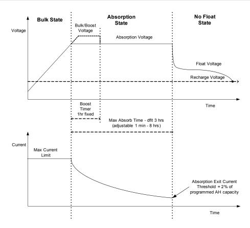
Figure 1-5 Two-stage Battery Charging Cycle
