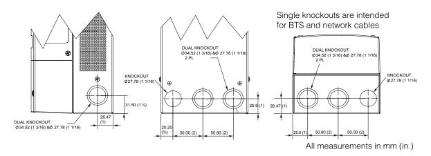
Figure 2-4 Knockout Dimensions
