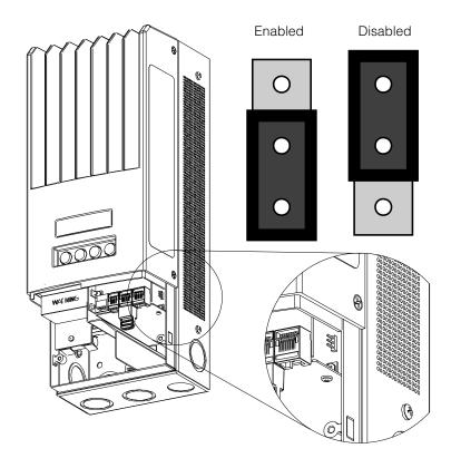
Figure 2-8 Jumper Location (CE Marked Model)
