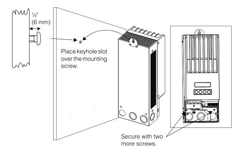
Figure 2-5 Mounting the Conext MPPT Solar Charge Controller
