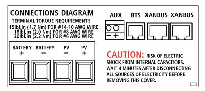
Figure 2-9 DC Connection Terminals
